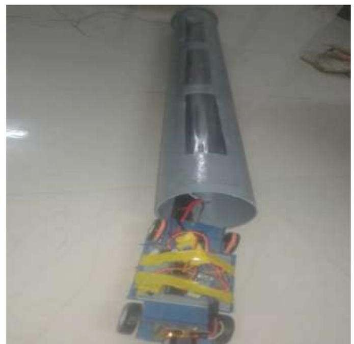
Figure 3: Hyperloop system with tube and pod
