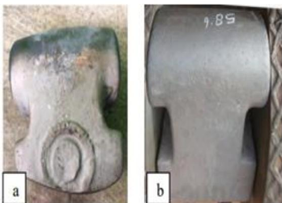
Figure 3: (a) Hammer crusher that is worn out, (b) hammer crusher that is still intact [16]
