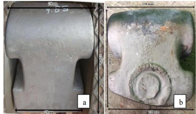
Figure 6: Hammer crusher (a) before wear (b) after wear [16]
