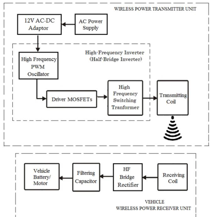
The receiving coil converts received electromagnetic field gain into high frequency ac current. Which is rectified by a bridge rectifier and given as dc output for motor of car or for charging.
