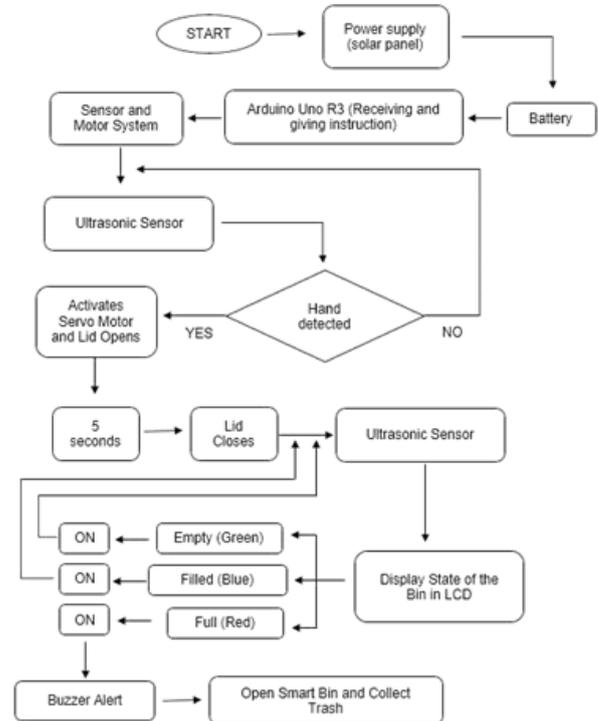
Figure 1: Conceptual Design of the Project
