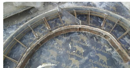
Figure 3: Preparing the Crack specimens (Ic1 and Ic2). (The drawing's dimensions are in meters)
