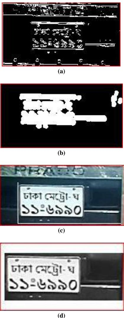
Figure 4: Images of different stages of Locating and Extracting Plate Area (a) After spatial differentiation; (b) After morphological operation locating white box region; (c) Initial image; and (d) Extracted image
