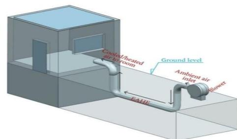
Figure 2: open loop system
