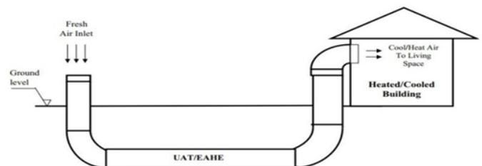
Figure 1: Open circle for space warming/cooling framework
