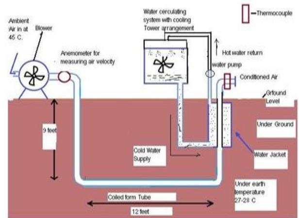
Figure 5: Experimental Setup of EAHE
