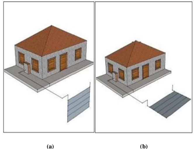
Figure 6: (a) - Vertical earth piping cooling VEPC system, (b) - Horizontal earth piping cooling HEPC systems
