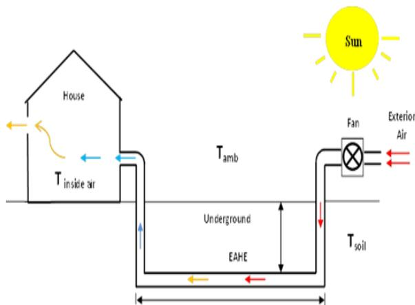
Figure 4: Air-ground heat exchanger in operation during the day and summer period
