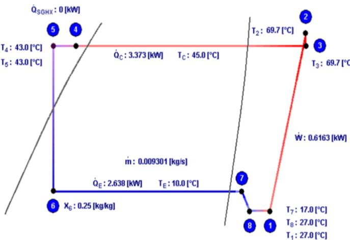
Figure 2: P-h diagram refrigeration cycle analysis
