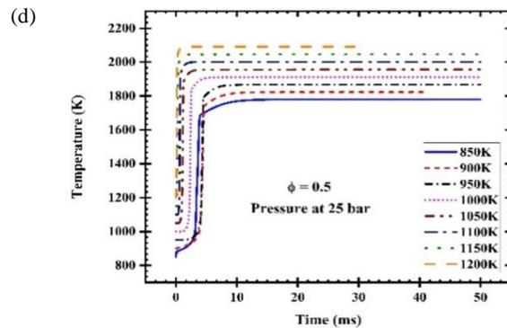
Figure 1: Shows the effect of temperature on the IDT at (a-b)  $\phi = 0.3$ , pressure = 20 bar and 25 bar. (c-d)  $\phi = 0.5$ , pressure = 20 bar and 25 bar
