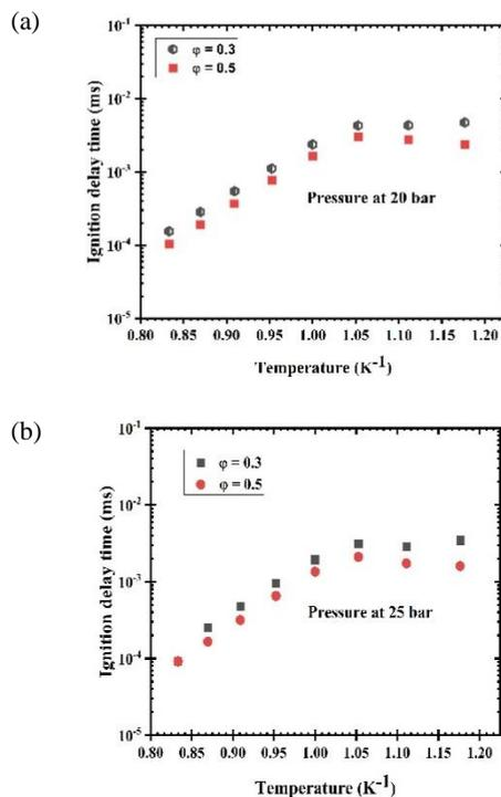
Figure 3: Shows the effect of equivalence ratio on the IDT at  $\phi = 0.3$  and 0.5, pressure = 20 bar and 25 bar
