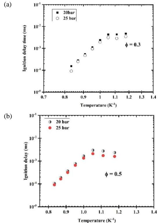
Figure 2: Shows the effect of pressure on the IDT at (a)  $\phi = 0.3$  and (b)  $\phi = 0.5$
