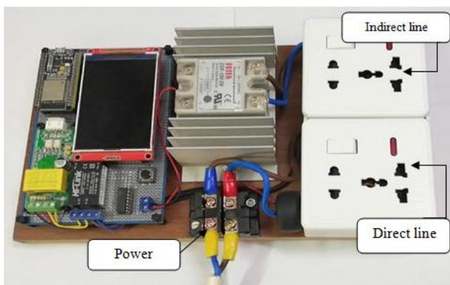
Figure 3: Shows the electronic design of the electrical energy measurement system
