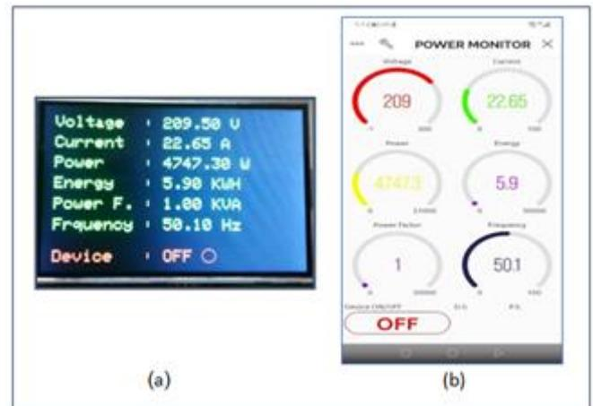
Figure 4: Shows the decision to turn off the indirect line after the current exceeds the specified value as (a) the system screen (b) Blynk application
