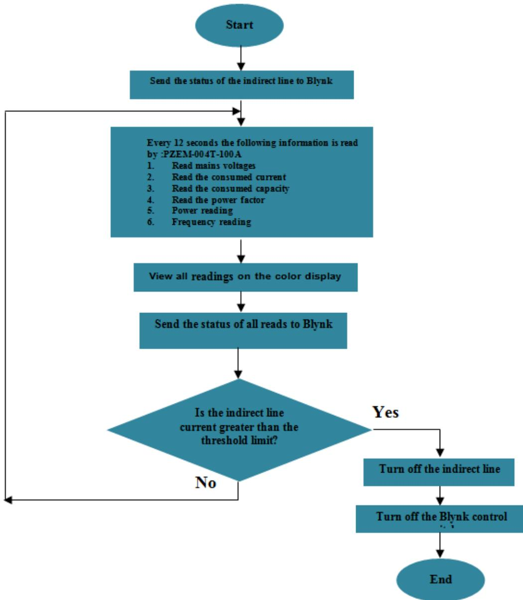
Figure 1: Flowchart for designing an electrical energy metering system
