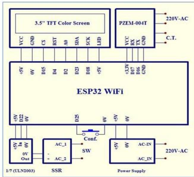
Figure 2: Electronic circuit design of the electrical energy metering system by ESP-32S Node MCU
