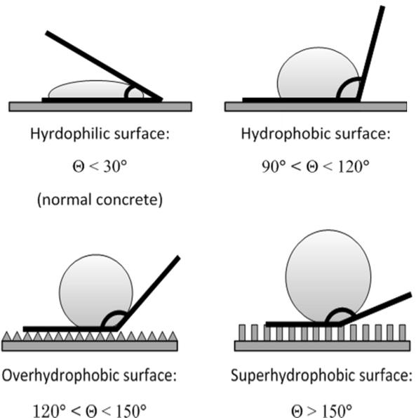
Hydrophobic and superhydrophobic material are surface protection materials and capable of increasing the angle of contact between the water droplet and the surface of concrete. Among various methods to protect concrete surface, impregnation of hydrophobic material is least harmful and highly efficient to inhibit capillary water absorption. It has been proved that hydrophobic agents could be effective for more than 10 years when applied as 6 months old concrete surfaces.
