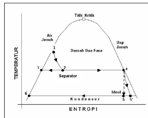
Figure 4: T-S diagram of GPP Single Flash Cycle (Saptadji M, 2019)
