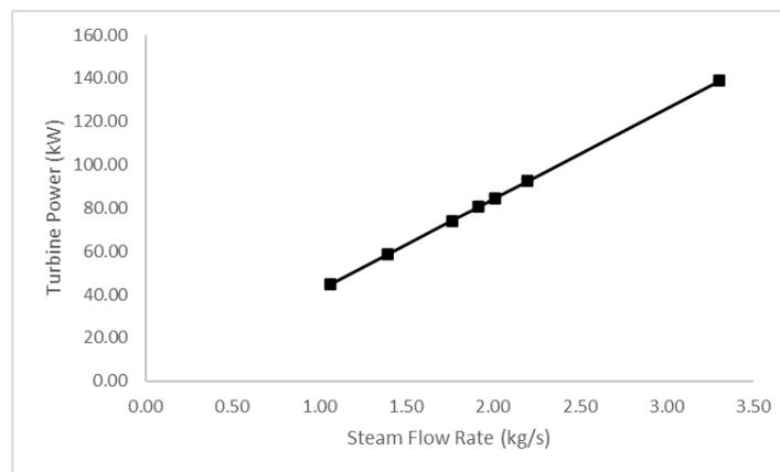
Figure 5: Steam turbine performance curve
