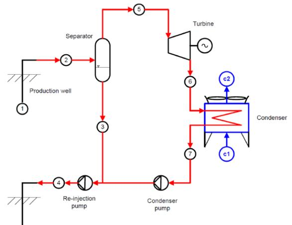
Figure 2: Single flash system in GPP (Valdimarson, 2011)
