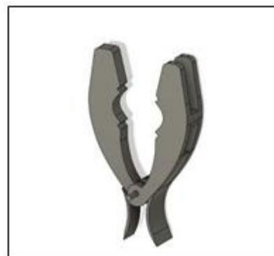
The spring is kept in tension by placing a rod of breakable material in between the jaws. The material can be made porous or can be externally weakened. It is done in such a way that the rod breaks on normal impact.
