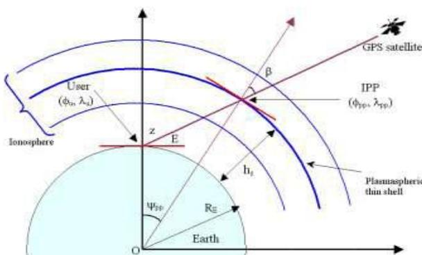
Figure 1: Geometry for the Conversion of Slant TEC to Vertical TEC (After Bolaji *et. al.*, 2015)
