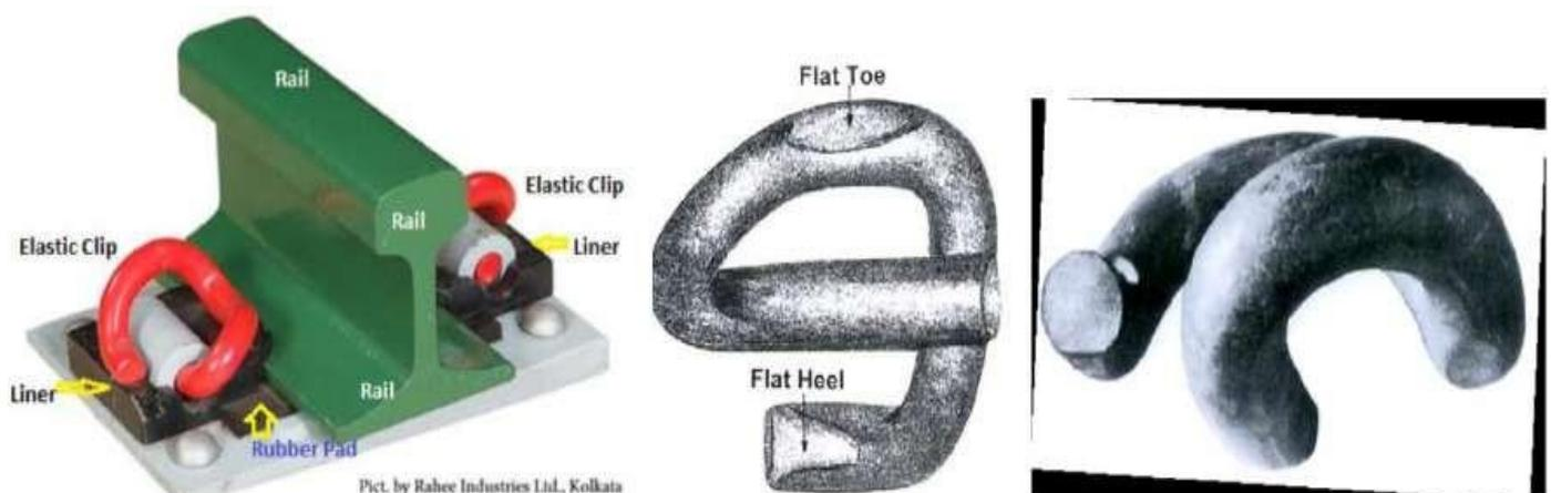
Figure 1.1 A schematic of Rail Track and Rail Fastening System
