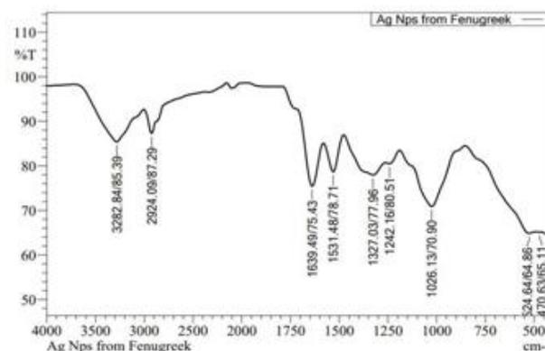
Graph 2: FTIR spectra of the AGNPs synthesized using the seed extract of fenugreek
