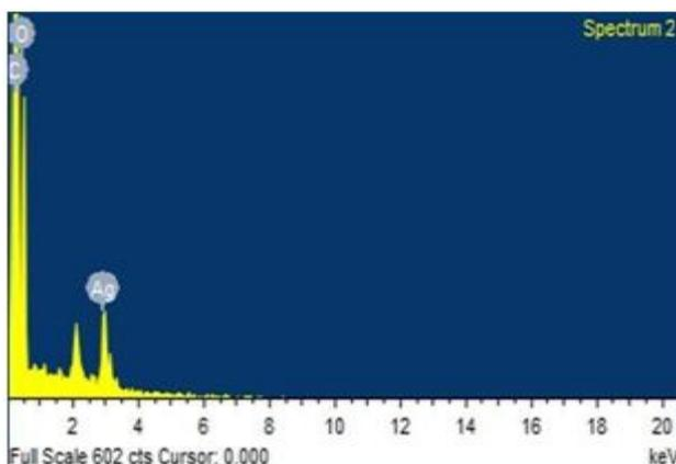
Graph 3: EDS spectra of the AgNPs synthesized using the seed extract
