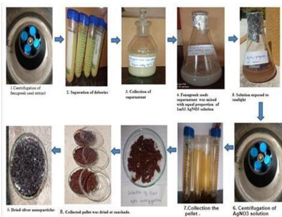
Figure 1: Overall process of Synthesis of silver nanoparticles
