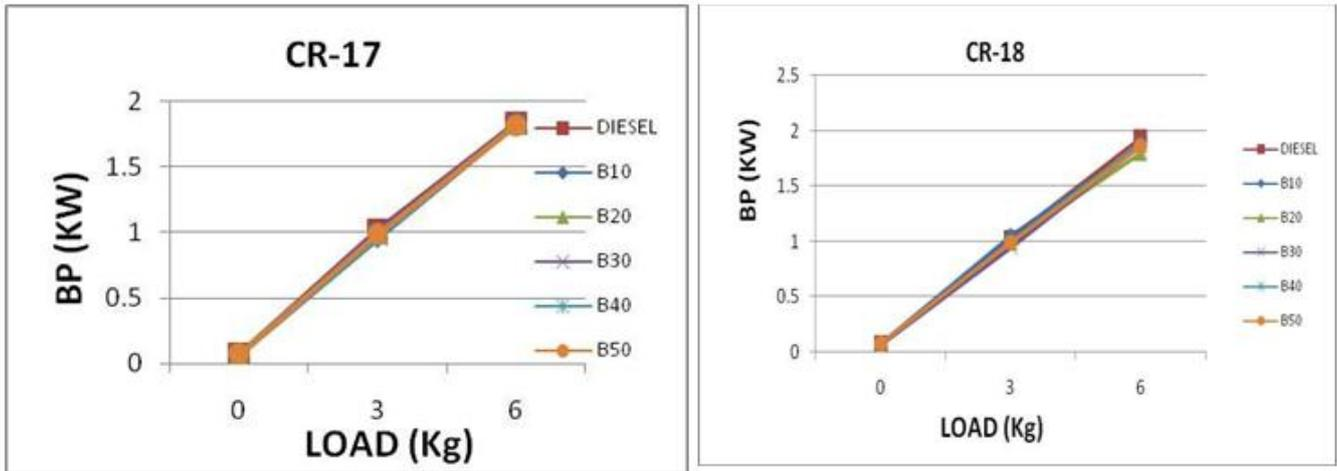
Fig. 2 BP vs Load for different Blends at CR 17 and 18
