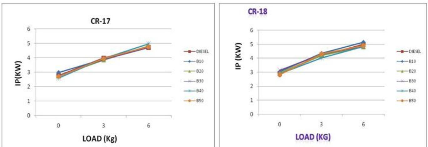
Fig. 4 IP vs Load for different Blends at CR 17 and 18
