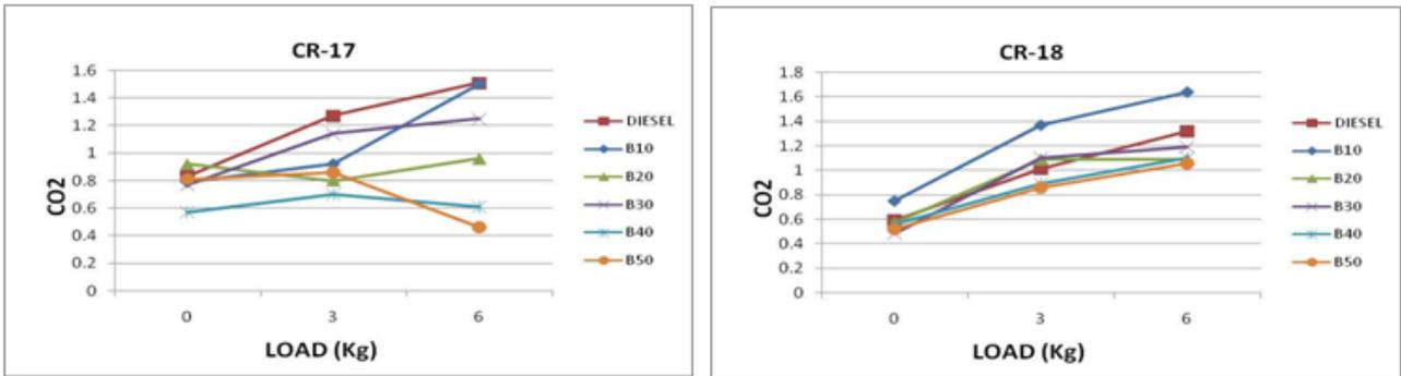
Fig. 8 CO<sub>2</sub> vs Load for different Blends at CR 17 and 18
