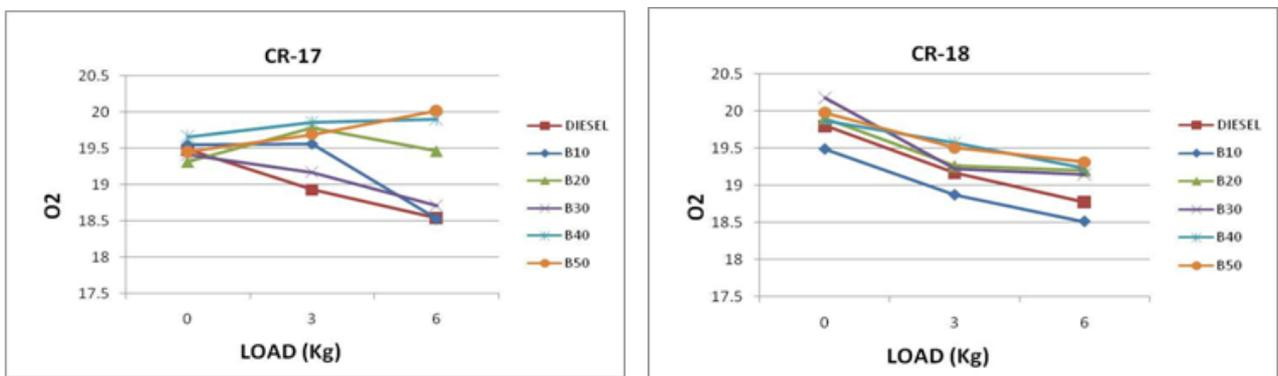
Fig. 9 O<sub>2</sub> vs Load for different Blends at CR 17 and 18
