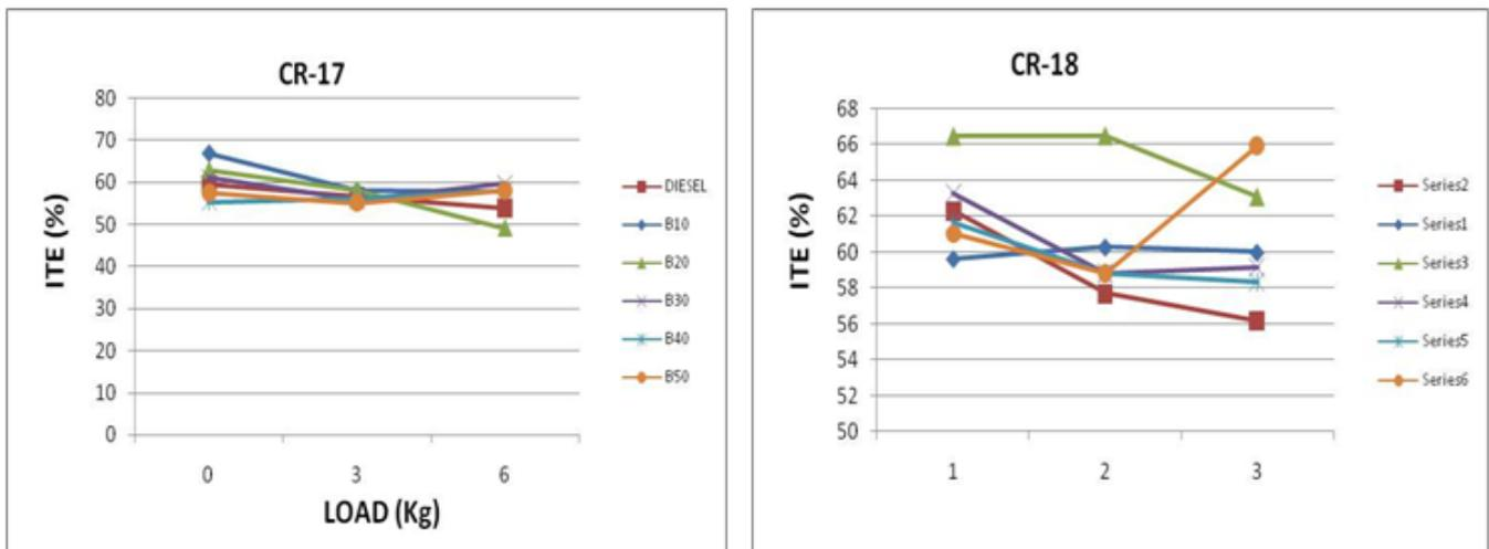
Fig. 6 ITE vs Load for different Blends at CR 17 and 18
