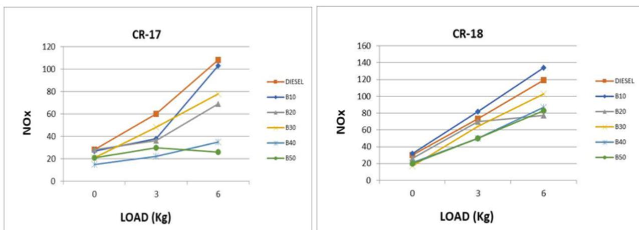
Fig. 12 NOx vs Load for different Blends at CR 17 and 18
