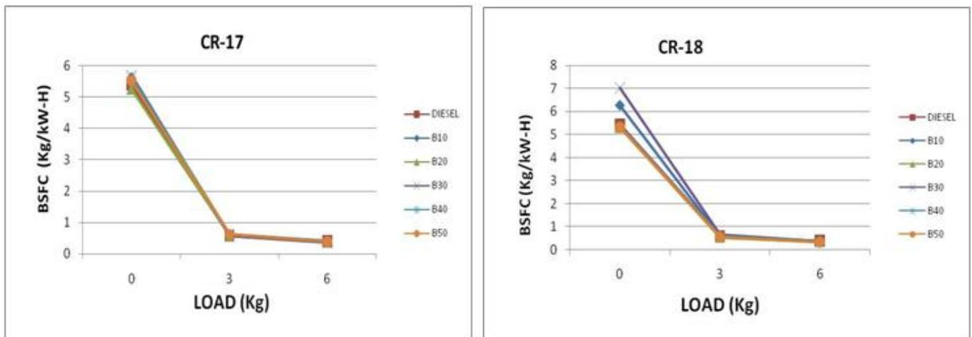
Fig. 7 BSFC vs Load for different Blends at CR 17 and 18
