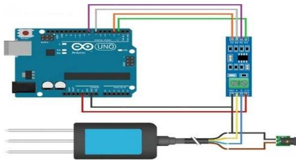
Figure 2: Circuit diagram of the IOT device
