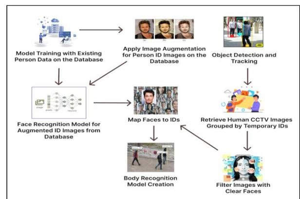
Figure 1: Integrated Human Proximity and Recognition System: Pre Deployment Environment Schematic
