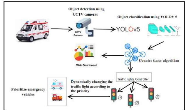
Figure 6 : Diagram of emergency vehicle detection
