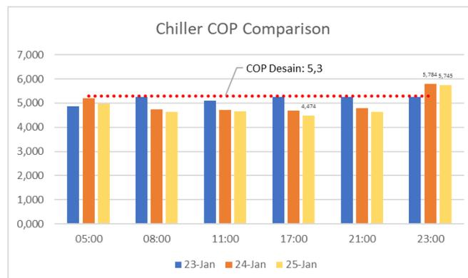
Figure 3: Comparison Chart of Actual COP with Design COP at 70% Part Load Condition
