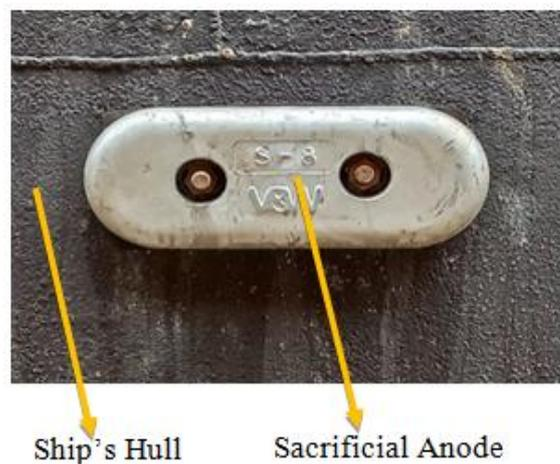
Figure 2: Ship cathodic protection
