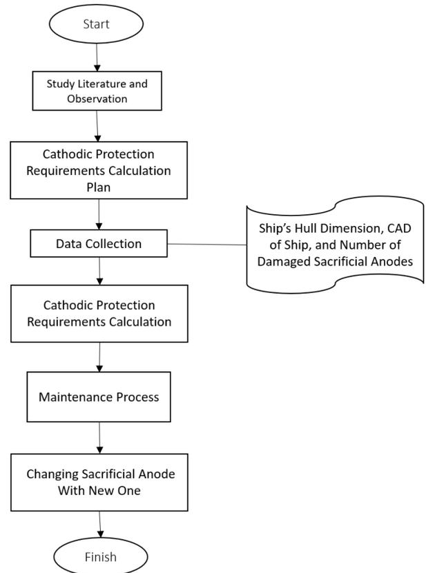
Figure 5: Flowchart of ship cathodic protection system maintenance procedure
