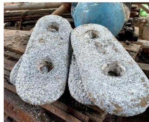
Figure 7: Rusted sacrificial anode
