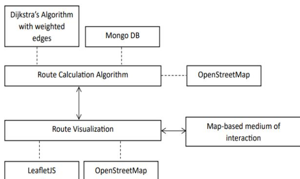
Figure 4: System diagram
