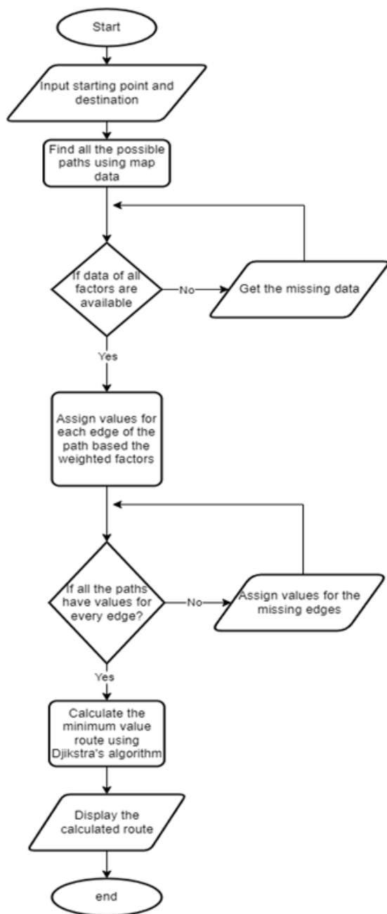
Figure 3: Algorithm Flowchart
