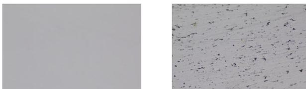
Figure 1: Surface appearance specimens before PWHT 100x magnification
