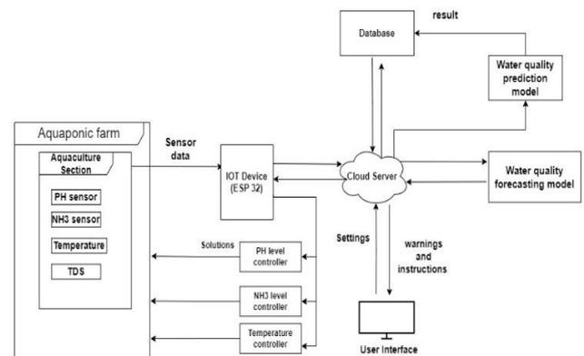
Figure 1: Process schematics of water quality control
