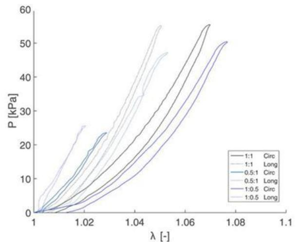
Figure 7: Biaxial experimental data behavior after preconditioning cycle at 1:1, 0.5:1, 1:0.5 ratios for pig colon tissue of pig (Ref : 14)
