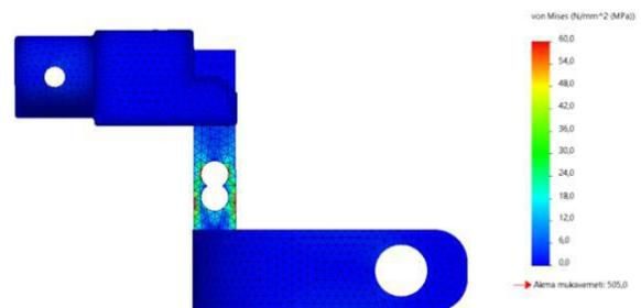
Figure 4: Von-Mises Stress under 200 N loading
