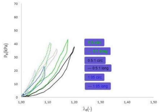
Figure 6: Biaxial experimental data behavior after preconditioning cycle at 1:1, 0.5:1, 1:0.5 ratios for small intestine tissue of a cow
