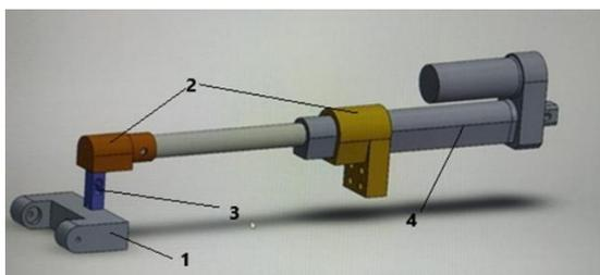
Figure 1: Fixtures components connected to the linear motor: 1.Specimen Grip, 2.Fixture components, 3.Load cell, and 4.Linear motor
