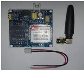
Figure 2.5: GPRS Shield Module SIM-900
