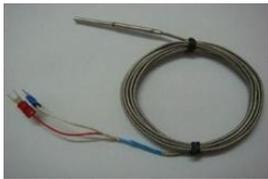
Figure 2.4: Thermocouple Sensor K-Type
