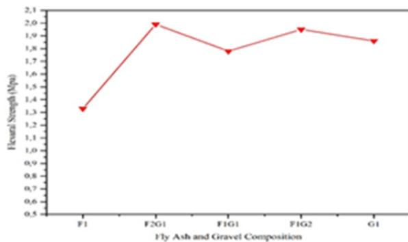
Figure 4: Flexural Strength Test Results
