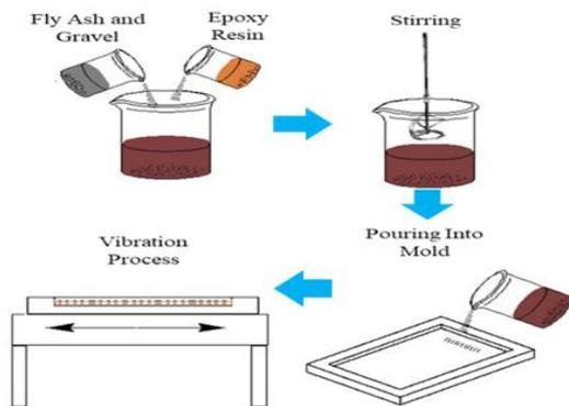
Figure 1: Manufacturing Process of Mineral Composite
