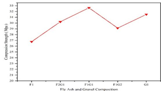
Figure 2: Compressive Strength Test Results
