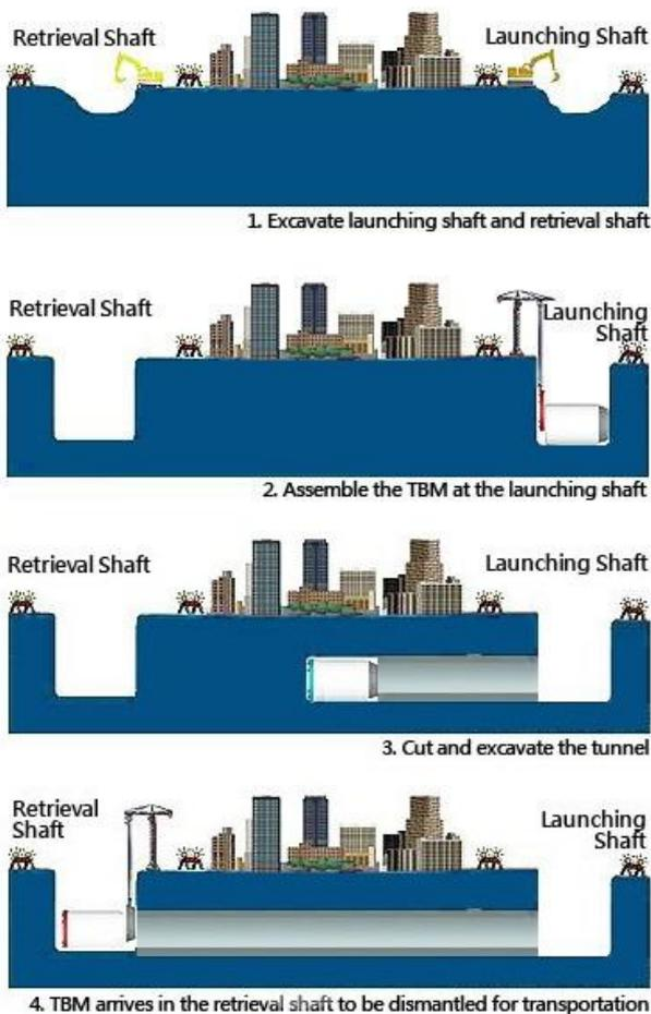
Figure 1: Shaft and TBM erection and movement (Source Railway Engineering)
