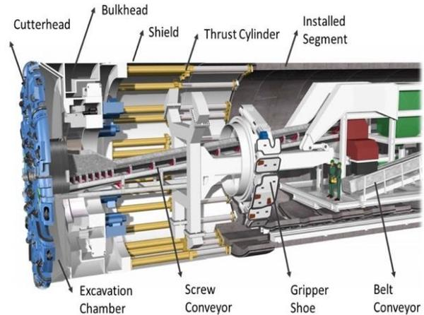
Figure 2: Tunnel Boring Machine (Source: TBM)
