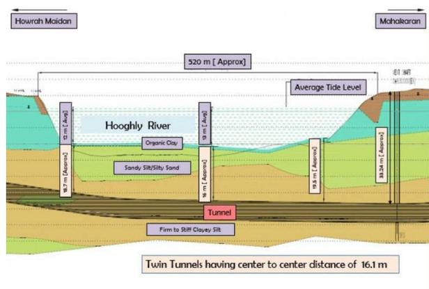
Figure 4: Tunnel cross section below river Hooghly
