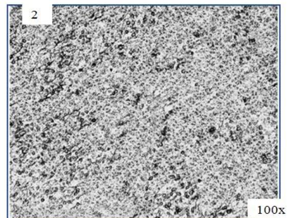
Figure 6.2: Microstructure Observation FSW 1400 rpm
