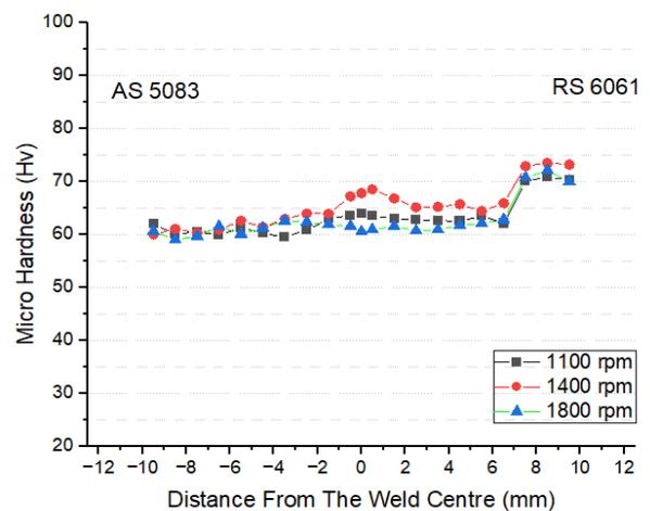
Figure 8: Chart of Micro Vickers
