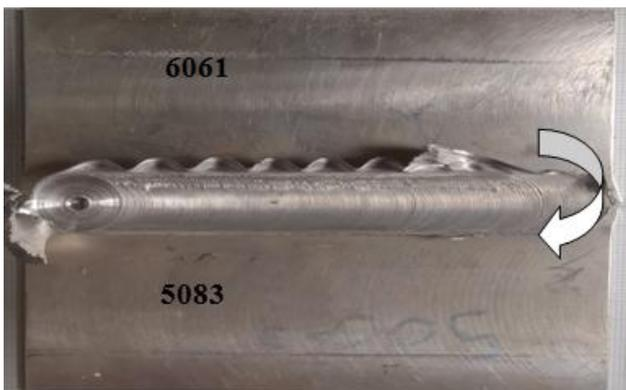
Figure 5: Result of FSW 1800 rpm
