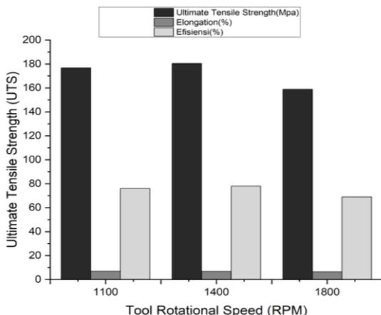
Figure 7: Chart of Tensile Properties
