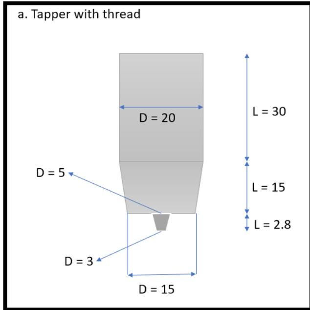
Figure 2: Design cylindrical tapered tool pin
