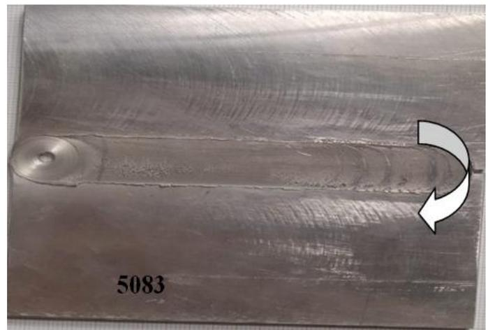
Figure 3: Result of FSW 1100 rpm
