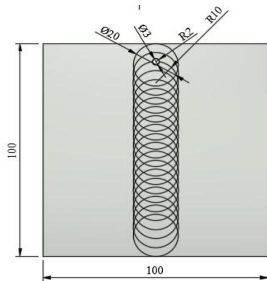
Figure 1: Schematic of FSW Welding Process for 5083-6061
