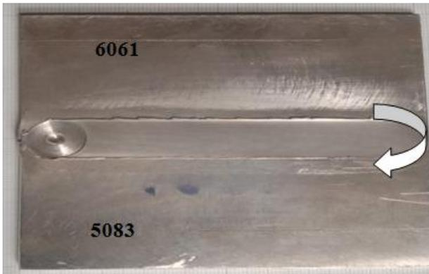
Figure 4: Result of FSW 1400 rpm
